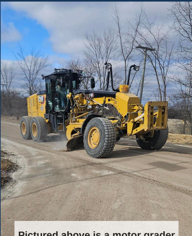
Pictured above is a motor grader in action!
